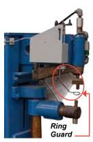
distance. At the start of each weld, the loop is sent downward before movement of the upper electrode. If the ring is stopped by a finger or other object before reaching the top of the part being welded, the limit switch does not trip and the electrode won't close.
