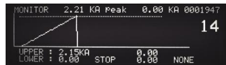
Monitor Screen – Shows weld current exceeding limit.
