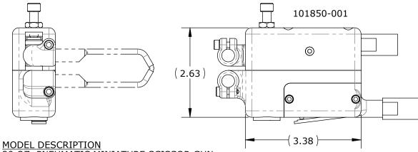
20 OZ. PNEUMATIC MINIATURE SCISSOR GUN. RIGHT ANGLED, WITH AIR COOLED CABLE S AND ADJUSTABLE STROKE. ELECTRODE PRESSURE = 15 LBS, AT 80 P.S.I.
