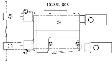
MODEL DESCRIPTION: 20 OZ. PNEUMATIC MINATURE SCISSOR GUN WITH WATER COOLED CABLES AND ADJUSTABLE STROKE. ELECTRODE FORCE = 15 LBS. AT 80 P.S.I.
