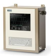
During each weld, Voltage, Current, Conductance, and Power profiles are automatically monitored. Force and Displacement profiles are available options to provide the most comprehensive weld quality monitoring. Any failed check results in an immediate alarm to alert production. The monitor records all data for future proof of weld quality without affecting production throughput.
